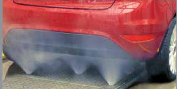
Two options are possible: static underchassis wash 10 bar [145.038 PSI], 90 L/min [19.8 gpm], and oscillating underchassis wash 15 bar [217.557 PSI], 120 L/min [26.4 gpm].
