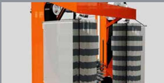
Micro-perforated curtains to prevent splashing during the wash process.
